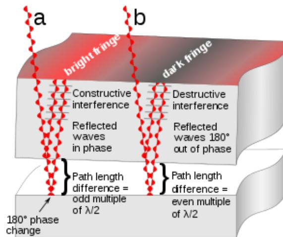
As discussed earlier, we see many reflection from the glass/air interference. We can neglect the fact that the glass is curved and believe that the reflection are collinear with in the incoming light (perpendicular to the air/glass interface) as seen in the drawing.
